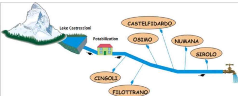
Fig. 3 - Potable water supply of Lake Castreccioni (obtained and modified from the Acquamambiente website)
