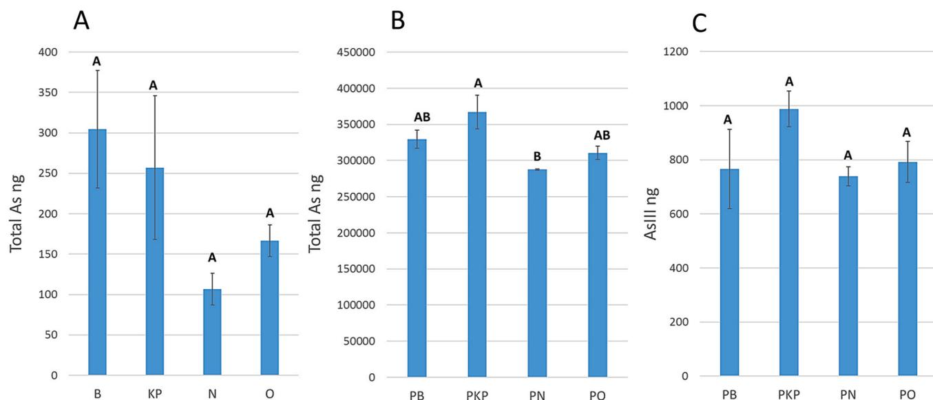
**Fig. 2.** Cumulated leached total As and AsIII. A: reference soil total As; B: polluted soil total As; C: polluted soil AsIII. KP: KP fertilizer; N: ammonium sulfate; O: organic amendment. P for polluted. Significance of differences between amendment conditions was evaluated separately for each incubation time using a non-parametric statistical method (details in material and methods section). Error bars represent the standard deviation of the means (3 replicates).
