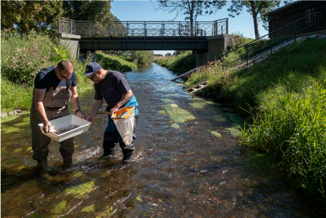
Surber sampling on the spot (0.25 m 2 ) scale; subsequent counting of EtOH fixed samples
