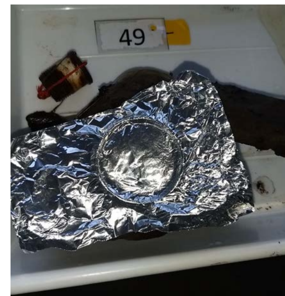
Oring and alufolie for area determination, important when surface is not flat
