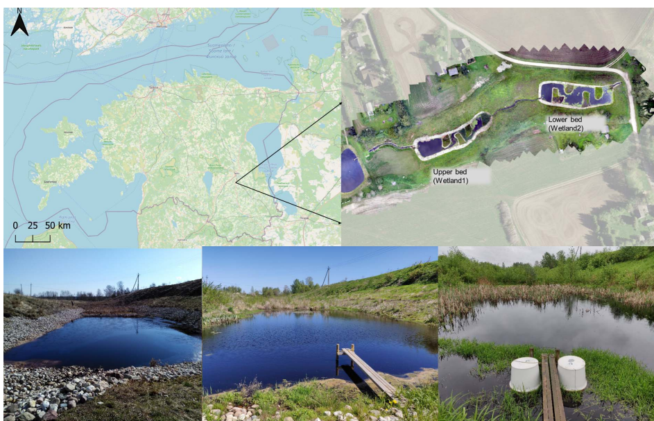
Figure 1. Vända in-stream FWS CW location in Estonia (top left); scheme of upper bed (Wetland1) and lower bed (Wetland2) (top right); and photos of vegetation development during different study periods (bottom from left to right: April 2017, May 2019 and May 2021).
