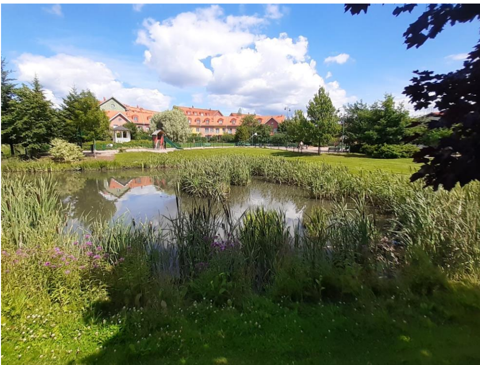
Figure 1. One of the ponds integrated to the neighborhood. They collect and hold stormwater to slow down the flowrate © Jussi Torkko
