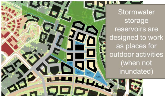
Figure 3.1. Stormwater management options in the Murrenpuisto basin
