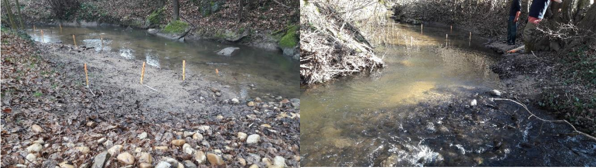
Figure 20. Wooden stakes with tape indicator to measure sand height. Near the porous barrier (left) and 30 meters upstream from the porous barrier (right).
