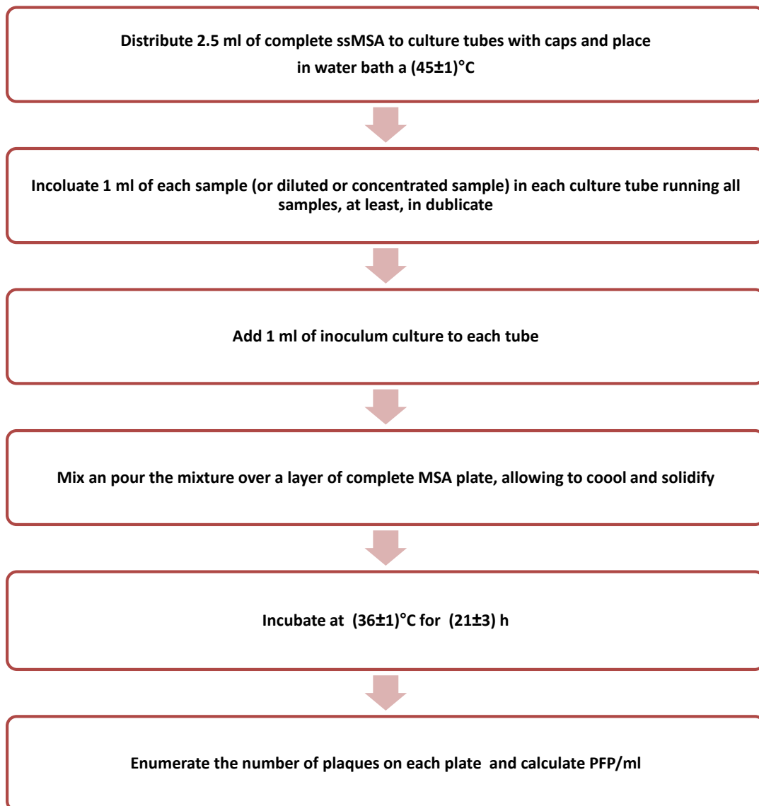
Figure 9: Scheme of the method for the detection and enumeration of somatic coliphages.
