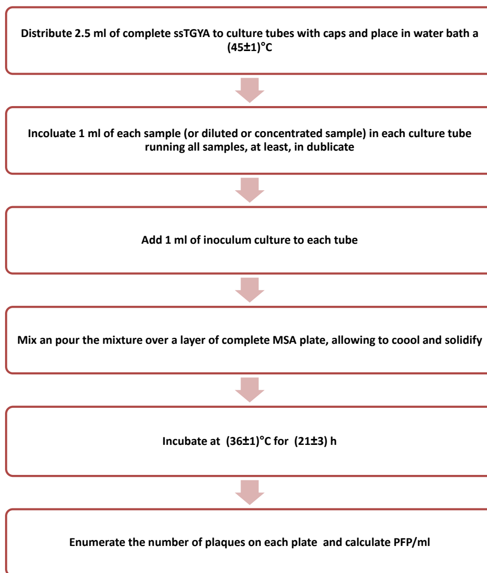
Figure 7: Scheme of the method for the detection and enumeration of F-specific bacteriophages
