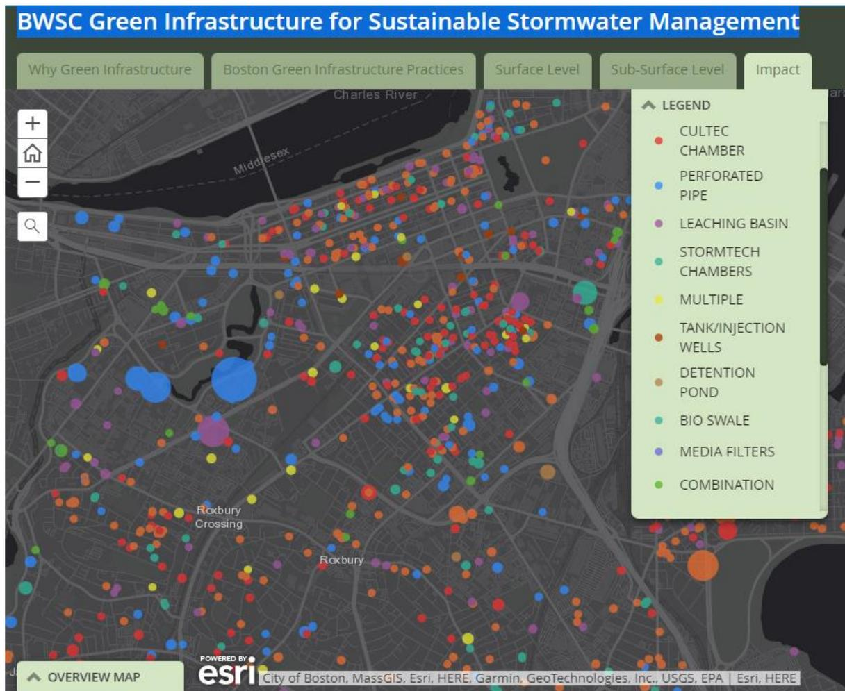
Figure 4. Map of green infrastructure installations in Boston. The size of each circle indicates the relative area that the installation can manage fir a 1 inch (approx. 25mm) rainfall event.
