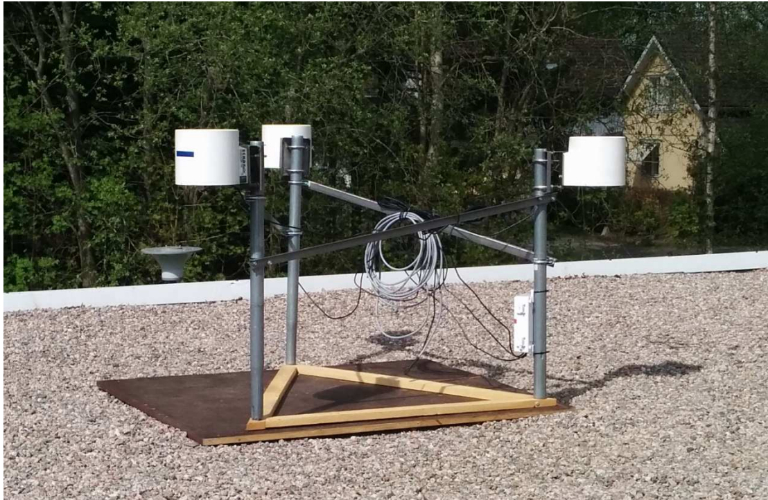
Figure 15. Three co-located on-site high-resolution tipping bucket rain gauges in Länsi-Pakila.
