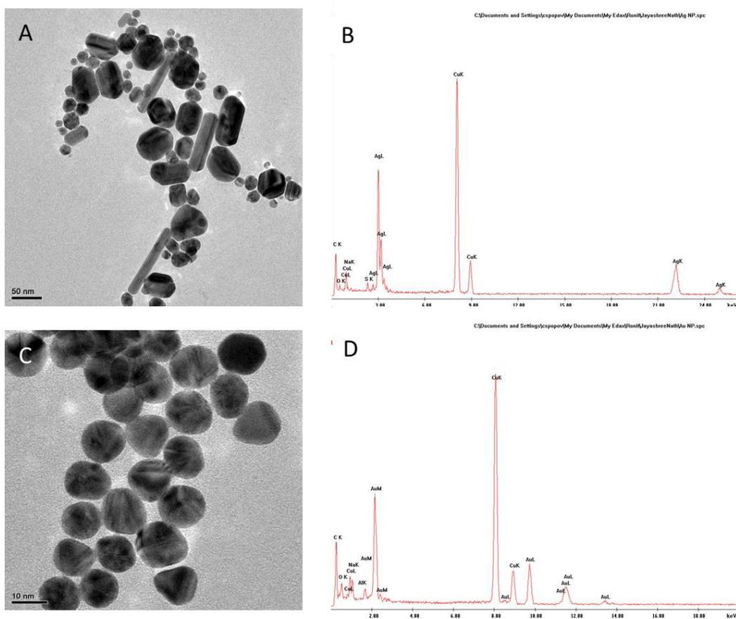
**Figure 1.** Transmission electron micrograph (A and C) and EDS analysis (B and D) of silver and gold nanoparticles, respectively.
