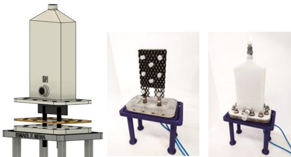
Figure 5. Ozone electrochemical cell investigated at UCLM at a bench scale.
