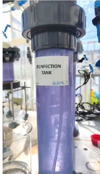
Figure 4: Disinfection tank with electrogenerated ozone gas fed into NF permeate.
