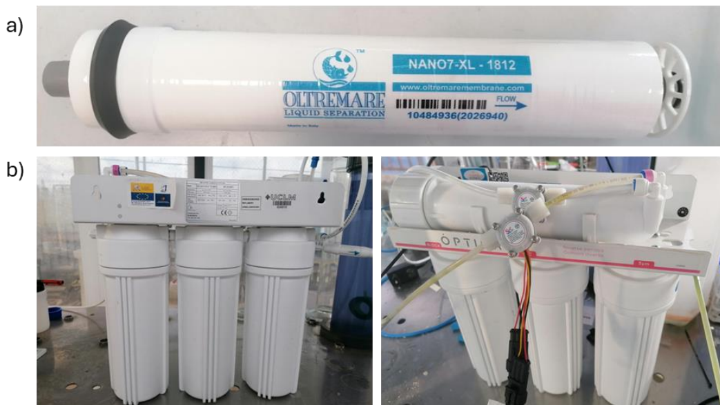
Figure 2: a) Nanofiltration cartridge and b) Filtration unit installed in the SERPIC prototype plant.
