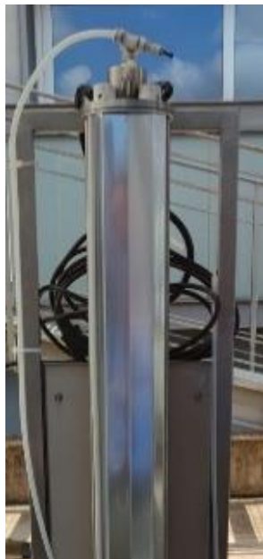
Figure 4 - Details for the (a) 3-sided geometry reflector bracket and dimensions; (b) photograph of the 3-sided geometric reflector enclosing the photoreactor prototype, and (c) reflectance values for MIRO®UVC aluminium reflector (source: technical brochure from Alanod).
