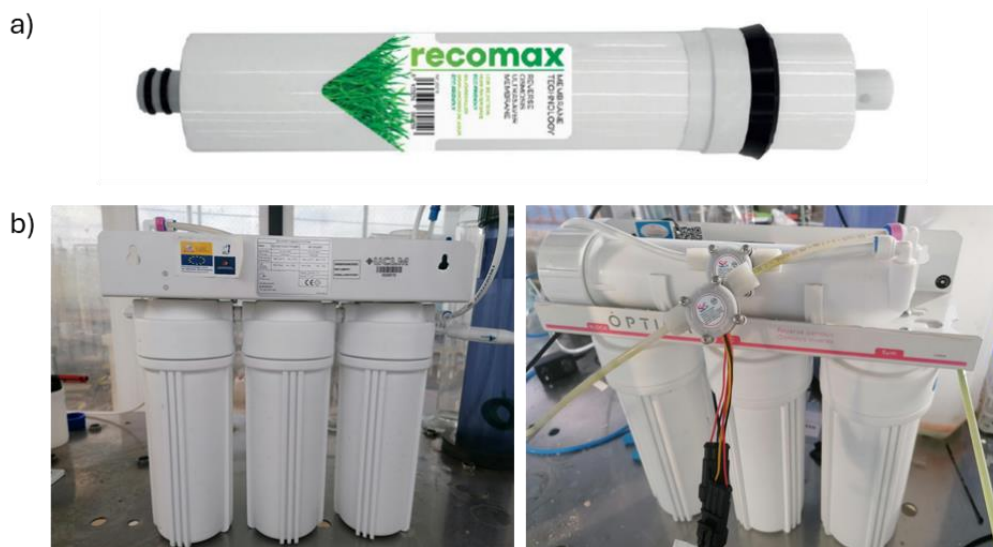
Figure 1: a) Reverse Osmosis cartridge and b) Filtration unit installed in the SERPIC prototype plant.
